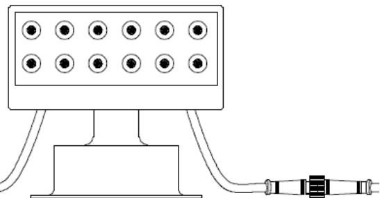
1.2 It's used for the DMX512 signal input and [power input cable](#) when testing for one PC sample or a series wall washer.
