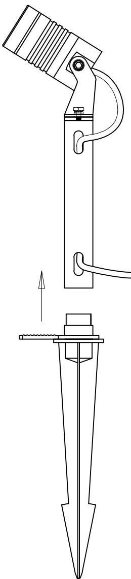
1.1 ,Screw out the screw from the pole.
